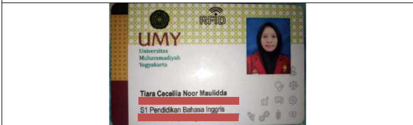
Figure 2. An example of student cards with the RFID tag used for the university entry
